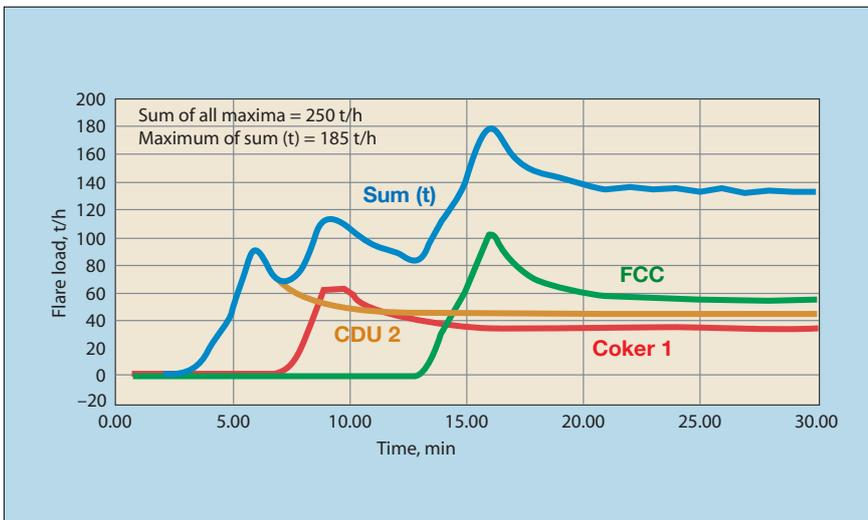
Figure 1 Simultaneity effects of a number of process units
