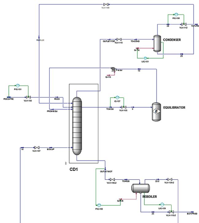
Fig. 1. Aspen HYSYS flowsheet of the dynamic cryogenic distillation column.
