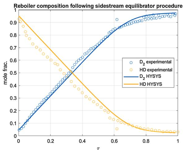
Fig. 2. Comparison of transient results between experimental and simulation data. The horizontal axis shows the dimensionless time parameter and the vertical axis represents the mole fraction of the mixture in the reboiler.
